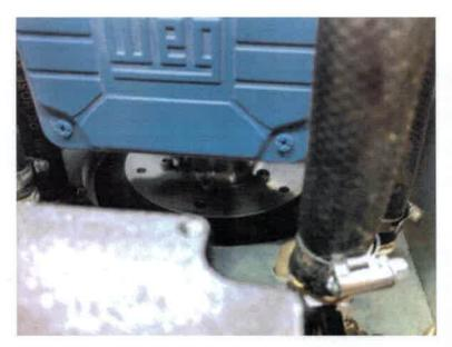
Image 7: 4 independent coolant outputs with a rear faucet each. They can be configured in the grinding so that two of them point at one end and the other two at the other end. Or on knives so that two point at the upper ends of the knives and the other two at the ends.
